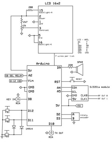
The Arduino can be powered from Vin or 5V pin
